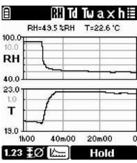
The graph clearly indicates when the readings have stabilized.
